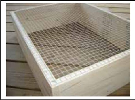
Once the wire mesh is stapled onto the frame of the screener you are ready to attach the 1 inch pieces of wood onto the bottom of the screener. These pieces of wood help keep the wire mesh secured to the screener and make sure the staple don't pull out when you're using it. {Don't forget to pre-drill your holes in the before screwing the 1 inch pieces onto the bottom of the screener}.
