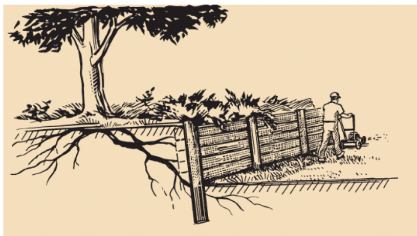
Figure 14. Crib walls can be used to limit the length of manufactured slopes, providing more room for trees and development.
