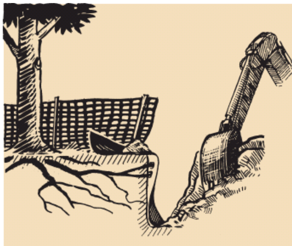
Figure 27. After roots are exposed and cleanly cut, the soil around them should be watered and covered with black plastic during hot periods. Large equipment can be used for mass grading after tree roots have been protected.
